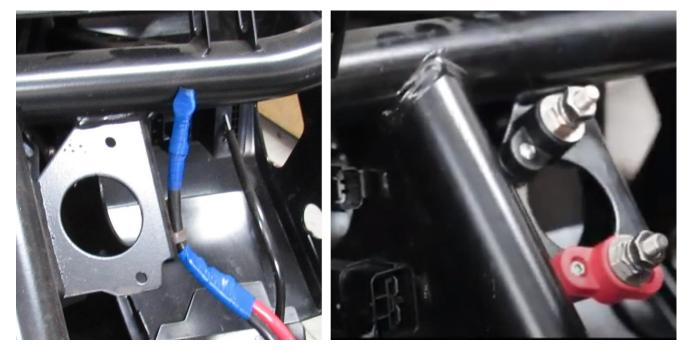
Install the ECU mount onto the center of the horizontal chassis tube under the most forward part of the dash using the included hose clamps. See below.
